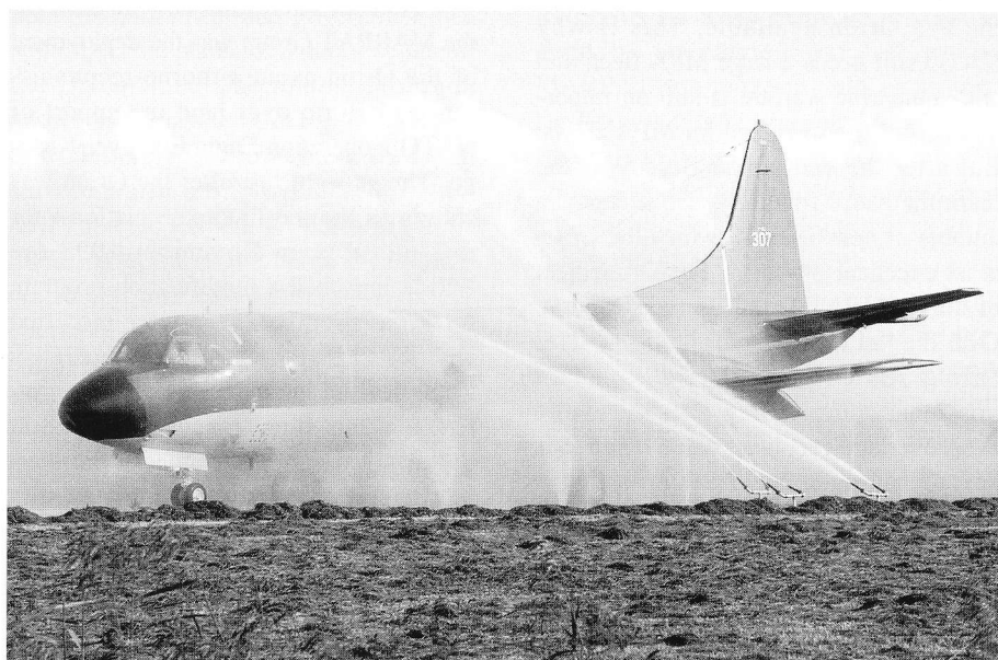
A RNLN P3C-III/2 Orion taxis through the rinse rack at RNLNAS Valkenburg (Marco Borst)
