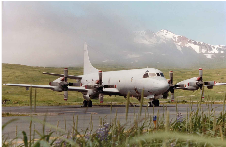
LEFT A fully unmarked P-3 Orion photographed by a crewmember of VPU-2 while on a detachment at a site in the North Pacific, some time in 1990. Again the AN/ALQ-78 ESM-pod in combination with the P-3B HF antennae identify this Orion as a special projects Orion. At the time of the picture VPU-2 was using both 154584 and 154585. (archive Jaap Dubbeldam) RIGHT Photographed landing at NAF Atsugi, Japan in December 2005 is P-3C Orion 160766, which is used by VPU-2 as a logistics aircraft. It is a rare example of a VPU-2 Orion showing both the actual last three of the BuNo as well as the badge of the squadron. (via Takafumi Hiroe)
