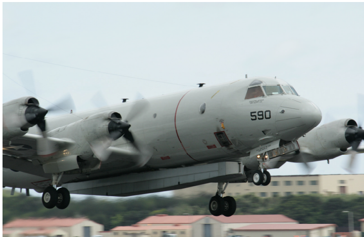
ABOVE LEFT - 161590 P3C BMUP+ operated by VP-1 departing Lajes on May 26th 2010 as "Navy YB590" while flying Rota-Patuxent River, showing to good advantage the Boeing antenna, hanging on the belly and the MWR system & the ARC-182 antennae (P-3 Orion Research Group) ABOVE RIGHT - A fine study of a P-3C BMUP+ without the LSRS pod. 161596 with VP-26 markings is taking off from NAS Brunswick on September 5th 2008 (photo by Jason Grant)
