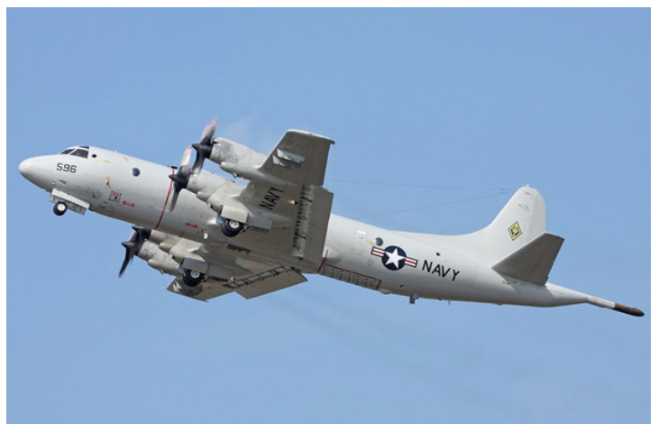
ABOVE LEFT - 161590 P3C BMUP+ operated by VP-1 departing Lajes on May 26th 2010 as "Navy YB590" while flying Rota-Patuxent River, showing to good advantage the Boeing antenna, hanging on the belly and the MWR system & the ARC-182 antennae (P-3 Orion Research Group) ABOVE RIGHT - A fine study of a P-3C BMUP+ without the LSRS pod. 161596 with VP-26 markings is taking off from NAS Brunswick on September 5th 2008 (photo by Jason Grant)
