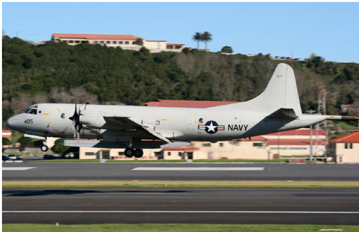
ABOVE LEFT - With the LSRS pod beneath the fuselage, P3C BMUP+ 161405 is seen about to declare "on deck" on December 6th 2007 as "Marlin00" at Lajes. ABOVE RIGHT - Orions with the LSRS pod are a rare sight for many of us. It is even rarer to see two of these photographed at the same time. This picture was taken at NAF Kadena in Japan in January 2011 and shows 161404 and 161586, both with VP-4 squadron markings.
