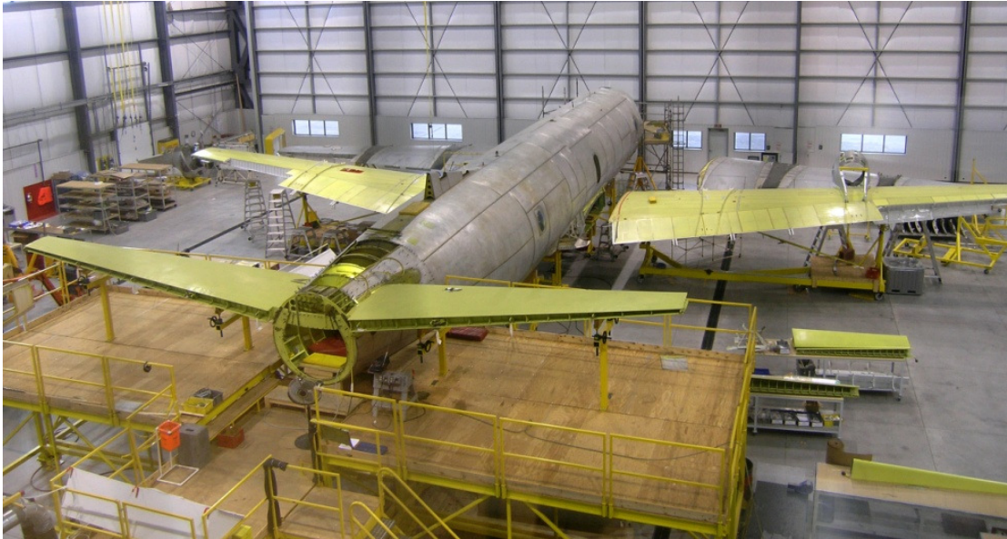
One of Norway's P-3N Orions is receiving its new wings at IMP Aerospace in Halifax, Canada. The airframe is over 40 years old, the new wings add another 20 years life time (photo: IMP)
