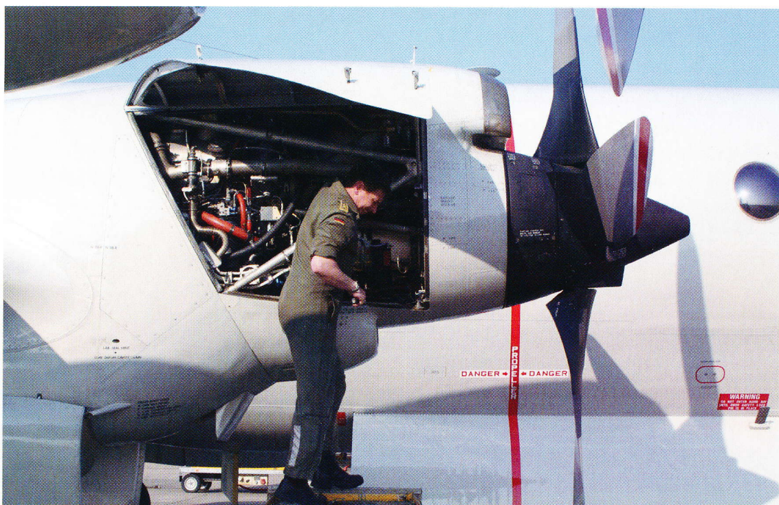
A German technician working on one of the P-3's Allison T-56 turboprops. The combination of greater reliability and longer periods between scheduled maintenance will give the Orion a higher availability.
